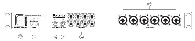
The remainder of the Scarlett OctoPre's inputs and outputs are on the rear panel.
