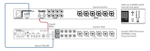
Here **ADAT OUT** on the Scarett OctoPre is connected to **OPTICAL IN** on a Scarlett 18i20 audio interface with a single optical cable. Both units are running at 44.1kHz sample rate. The OctoPre's **WORD CLOCK IN** input is connected to **WORD CLOCK OUT** on the Scarlett 18i20 with a BNC cable and the OctoPre's clock source is set to WORD CLOCK. The 18i20's clock source is set to INTERNAL (via Focusrite Control), thus making it the sync master.
