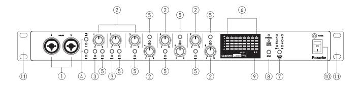
All operational controls and metering for all eight channels are on the front panel.
