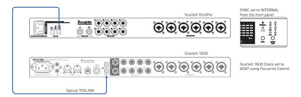
Here **ADAT OUT** on the Scarlett OctoPre is connected to **OPTICAL IN** on a Scarlett 18i20 audio interface with a single optical cable. Both units are running at 44.1 kHz sample rate. The OctoPre's clock source is set to INTERNAL, and the 18i20 is synchronised to it because its clock source is set to ADAT (via Focusrite Control).
